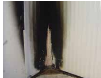
End of test showing minimal panel damage
