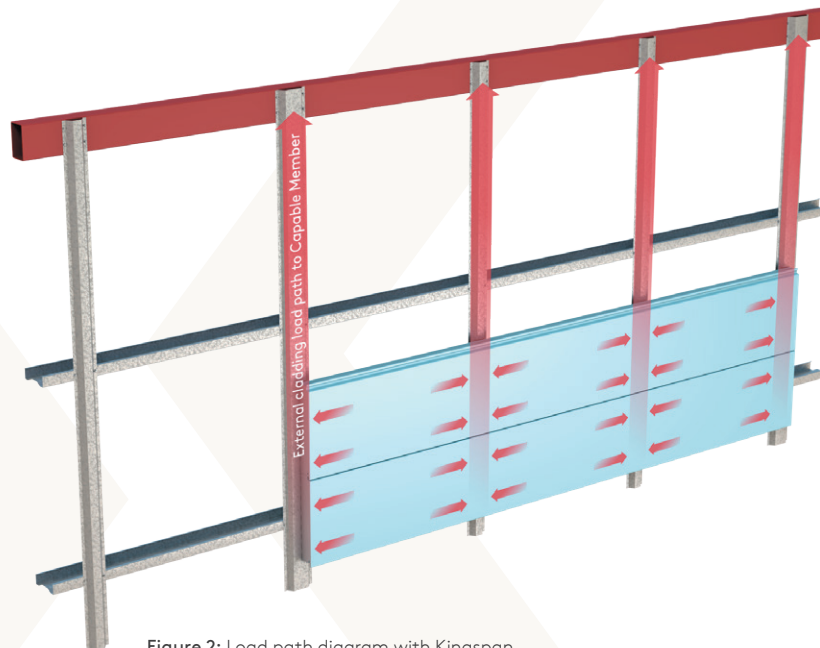
Figure 2: Load path diagram with Kingspan QuadCore® AWP Wall Panels.
